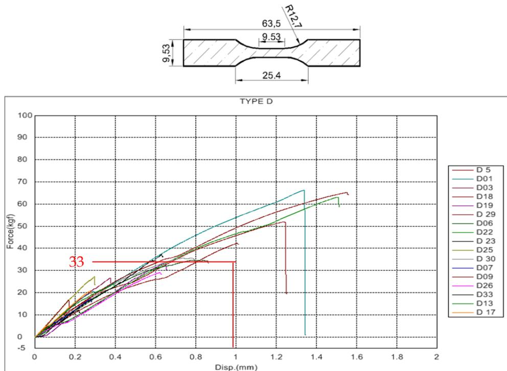
Fig. 8. Type D fiber Angle between 0-5°
