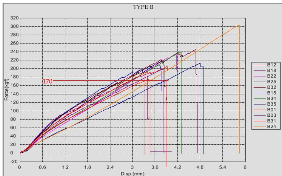
Figure 4: TYPE B fiber Angle between 8-17°
