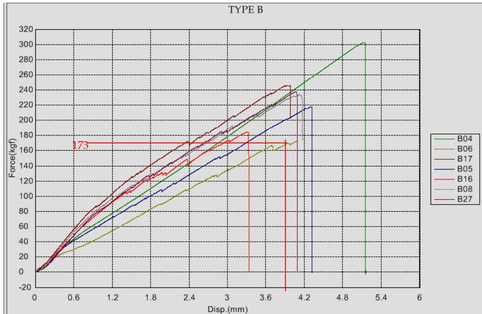
Figure 3. TYPE B fiber Angle between 0-7°
