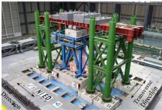
Fig. 3 C1-6 column experiment set-up using E-Defense shake table
